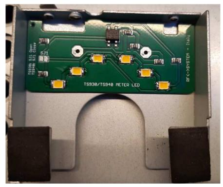
Solder both cutted wires (the polarity does not matter) on the solder pad from the backside of holder frame:
