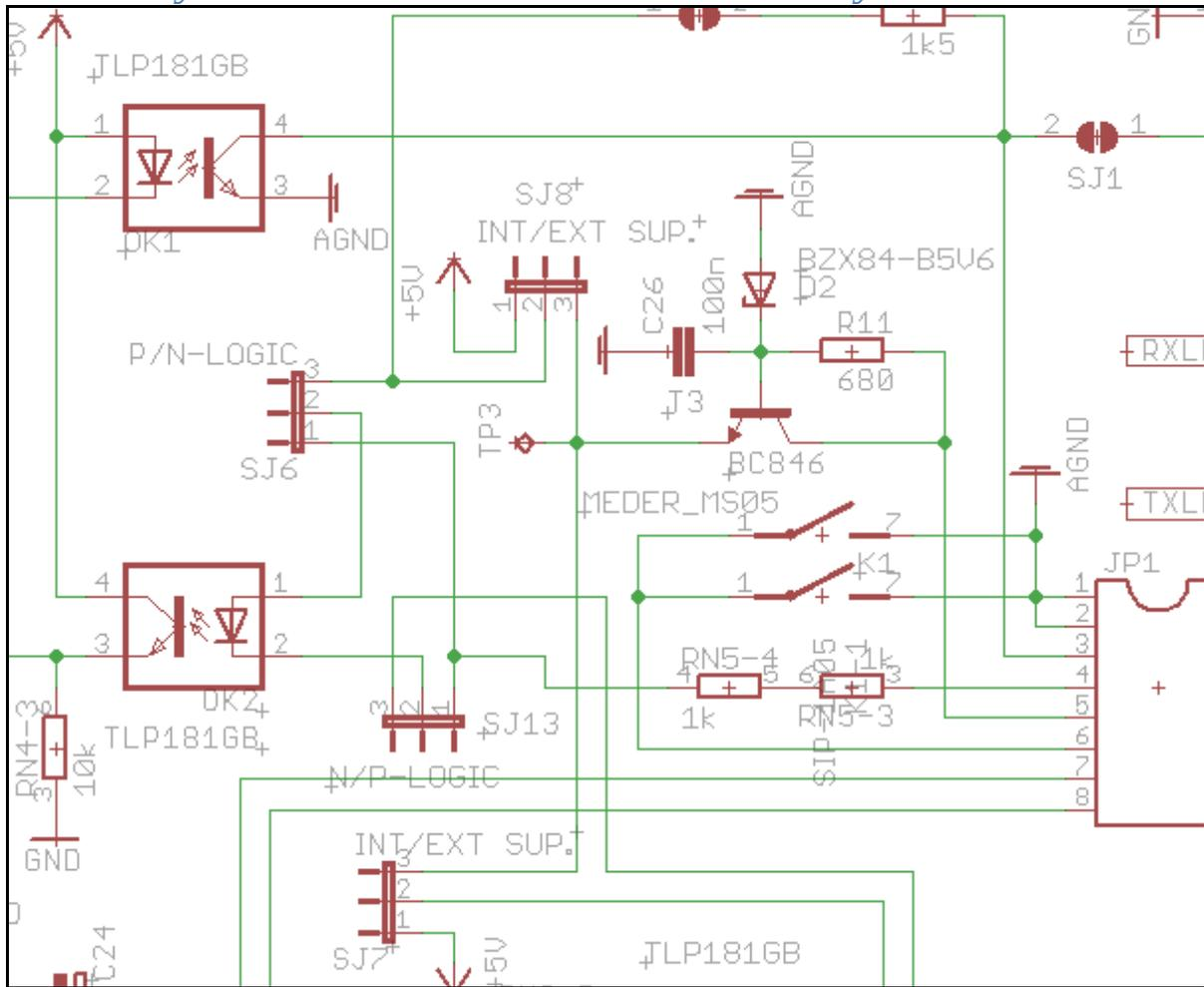
**CW / FSK Pull-up and SQL (COR) negative logic supply source (SJ8)**
