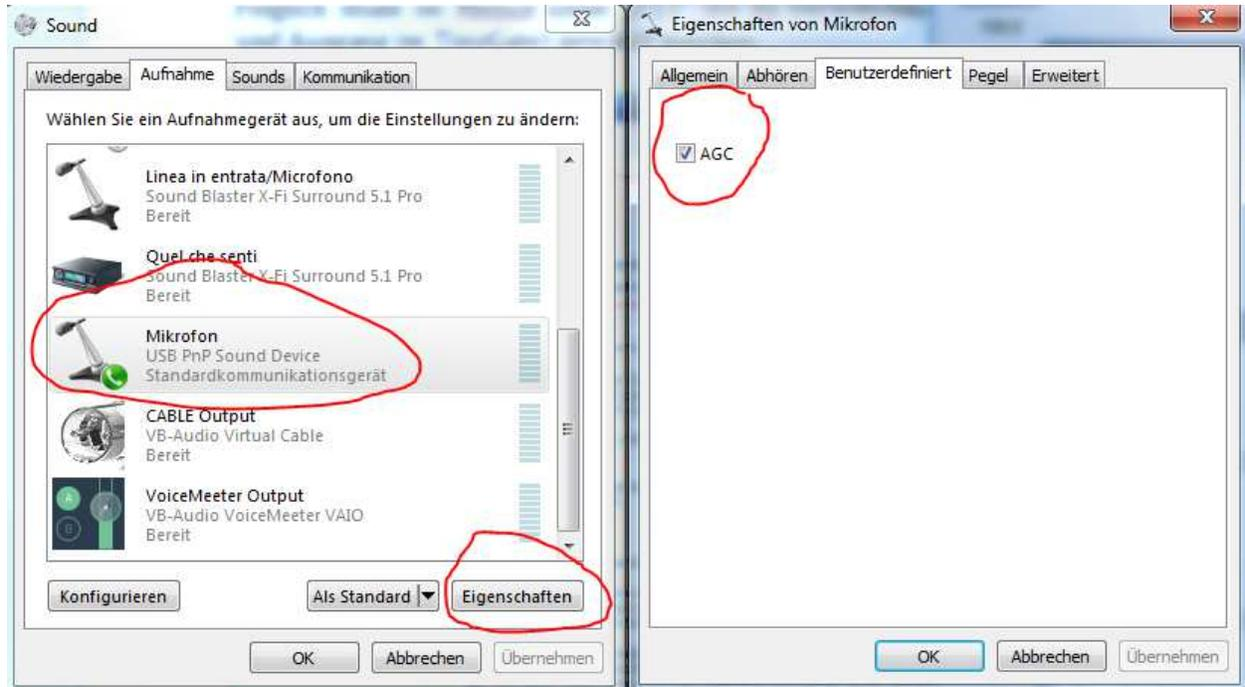
In any case it is advisable to deactivate the preamplifier first and controlling the audio output level of the transceiver. Only if this was not sufficiently high despite the “RX” potentiometer being at maximum, then one may try and activate the preamplifier with “AGC”.
