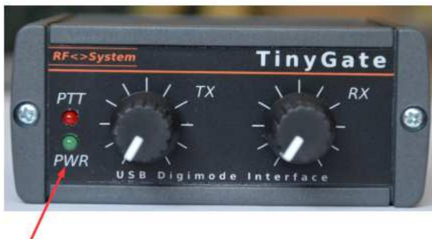
**Note:** the green LED "PWR" on the front panel flashes when a software application accesses the TinyGate audio interface. **The "PWR" LED remains off until the operating system starts up and the relative audio drivers are loaded.**
