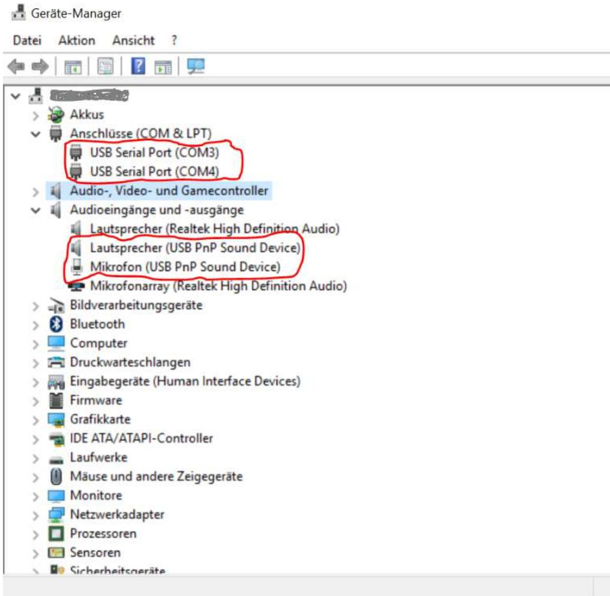
It is useful to note that the progressive numbering of the two serial ports (COMx) depends on the PC and operating system, so it is possible that this should differ from PC to PC.
