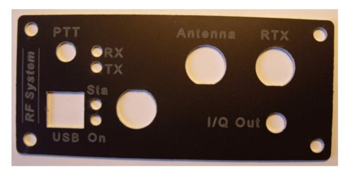
2 - Rear panel for a to be assembled PMSDR (do not assembly the BNC-connector on the PMSDR-board)
