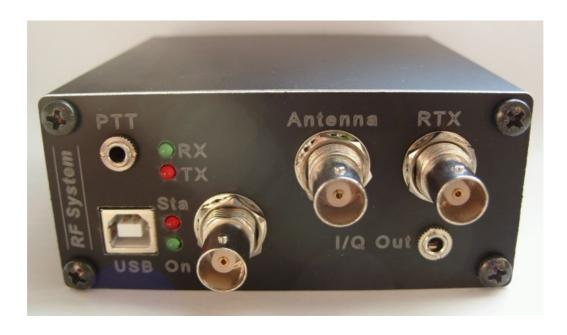
2 - Rear panel for a to be assembled PMSDR (do not assembly the BNC-connector on the PMSDR-board)
