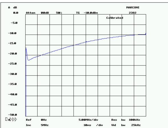
**Fig. 173: Return Loss Input without Prefilter (pass-through)**
